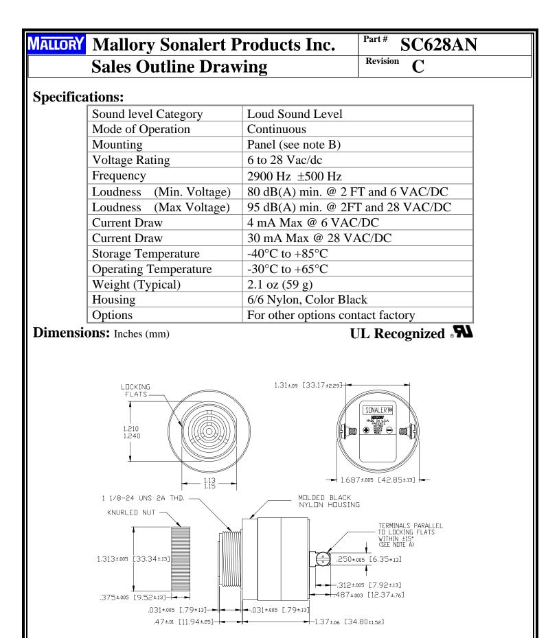
NDTE A: TERMINALS-.032 BRASS TIN PLATED, TAPPED FOR #6-32 SCREW. TWO #6-32 NICKEL
